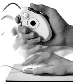
can be steadied by holding the mouse motionless for a few seconds. The trick is to relax and hold the GyroPoint just like you were shaking someone's hand.
